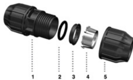
1. BODY - Polypropylene PP-B 2. O-RING - Nitrile Rubber NBR 70 3. INSERT - Polypropylene PP-B 4. SPLIT RING - Polyacetal 5. NUT - Polypropylene PP-B
